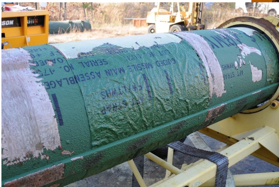
MMA Feed System with Leak Signature
