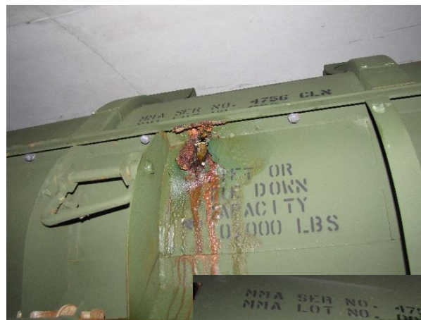
MMA Container with Evidence of Nitric Acid Release
