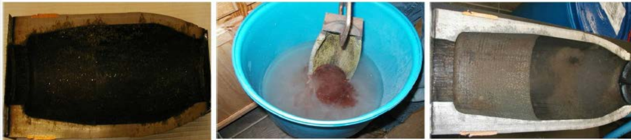
Rapid decontamination of halved bomb casings before and after MuniRem ® treatment
