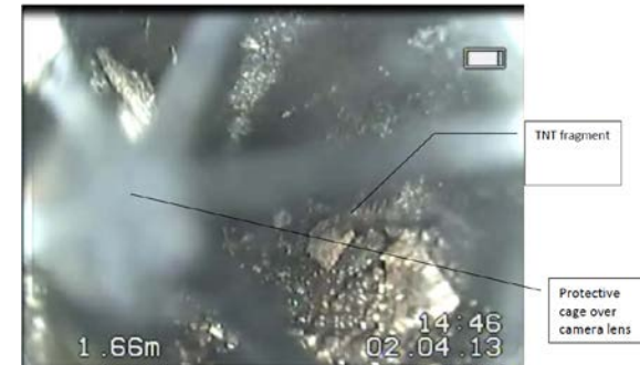
Inside of the explosive hazard pipe before treatment
