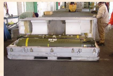
USAF Cluster Bombs – FZU-39 Altimeter fuzes, CB411 containers
