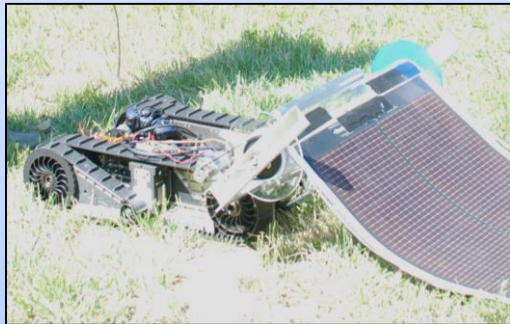
Deploy Panel & Charge Batteries
