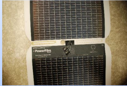
Panels are sewn into a single strip and then wired
