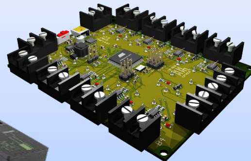
Power distribution board
