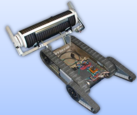
Solar panel is stowed on rotating drum
