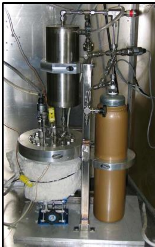
Semi-Continuous reactor with storage tank 4L open volume (rate: 10L H 2 /hr for 8 hrs)
