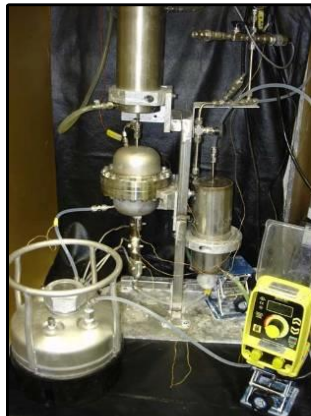
Continuous reactor producing H 2 (rate: 100L/hr as long as needed)
