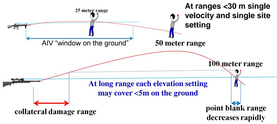
Each velocity setting may cover 25-30 meters, but at long range 2 to 6 elevation settings may be required for each velocity setting.
