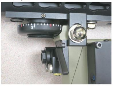
Range target, electromechanically select muzzle velocity, electromechanically adjust NL weapon elevation regulating NL Point of Aim co-incident with Lethal Point of Impact
