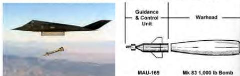
Figure 1: General Purpose Weapon Delivery with Laser Guidance
