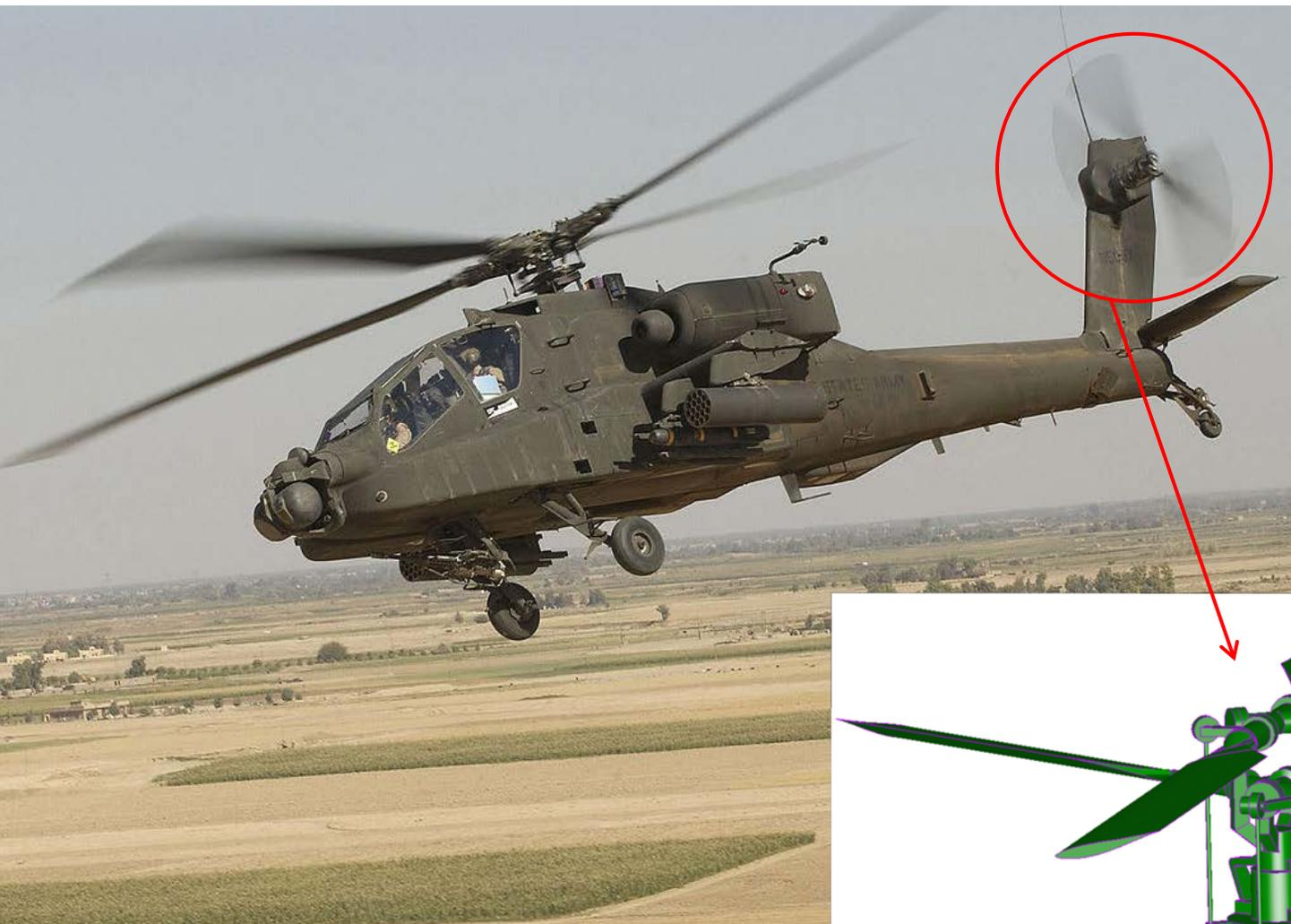
Apache attack helicopter is equipped with a teetering, stacked, scissored tailrotor configuration
