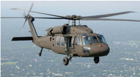
**Context:** The Army is studying the impact of increasing engine power on legacy rotorcraft. An increase in power available will allow the rotorcraft to hover at higher/hotter/heavier conditions. However, a consequence of this increased capability is that the tail rotor may not have sufficient thrust to maintain directional control of the helicopter.
