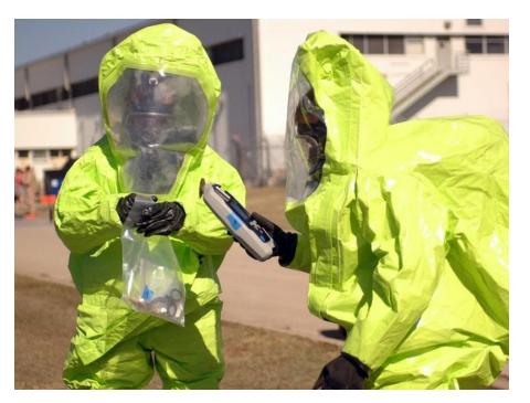
Soldiers participating in the toxic industrial chemical protection and detection equipment training, use an Ahura Scientific FirstDefender to identify chemical agents, Nov. 18 2009, at Fort Hood, Texas. The handheld device uses Raman spectroscopy to identify a wide variety of chemical substances, from common household items to deadly industrial toxins. (www.Army.mil/protection detection equipment hazmat)
