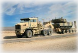
Heavy Equipment Transporter (HET)
