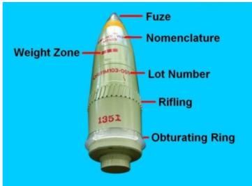
(3) Cartridge, 120mm Mortar EFSS
