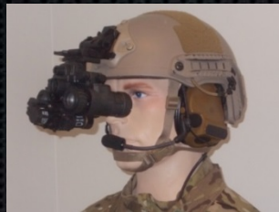
Night Vision Goggle w/ Clip-on Thermal Imager
