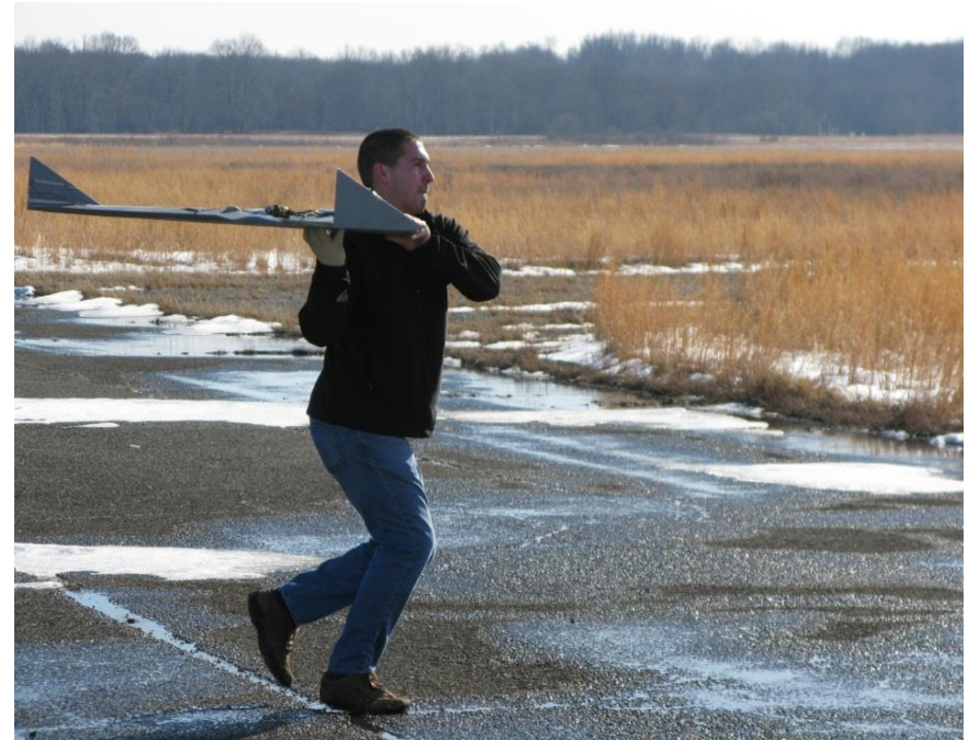
Hand launch of the Procerus research AUV controlled by JHU/APL's Autonomy Tool Kit (ATK)
