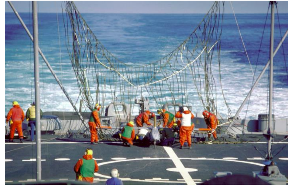
Crewmen recover a RQ-2 Pioneer UAV from the deck of the USS Iowa (BB-61), 1986
