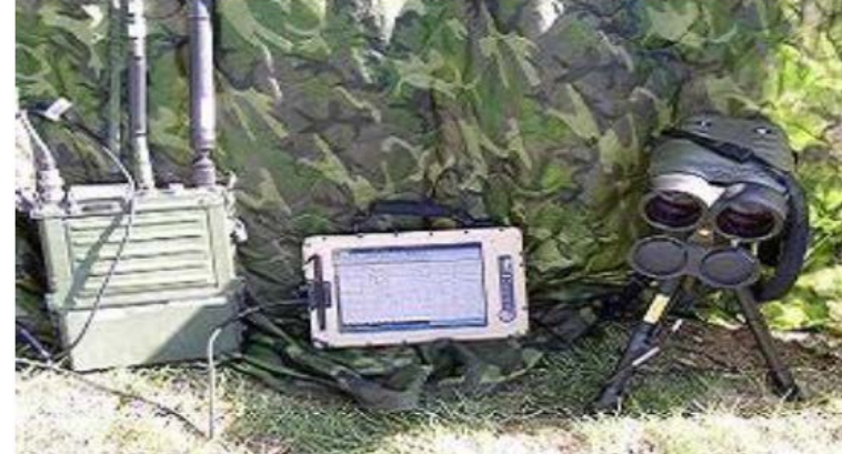
The FO's modern method: Target Location, Designation, and Hand-Off System (TLDHS)
