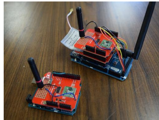
Arduino Active RFID RM and Sensor Device proof of concept
