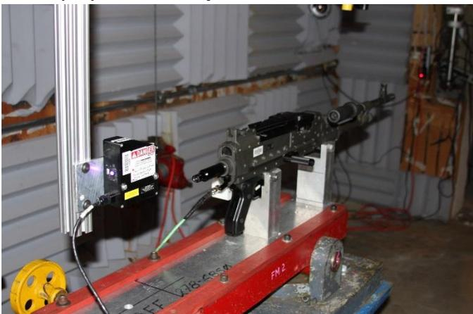
(U) Nylon bolt adapter for laser location
