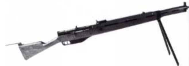
Rossignol 1901 ENT B1 “Automatic Rifle” @ 21.3 lbs Direct Gas Impingement / Rotating Bolt / Select Fire.
