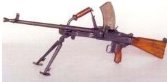
Cz Vz 52 LMG – Rear grip slides forward and back to charge 7.62X45mm & 7.62X39mm Mag. or Belt feed.
