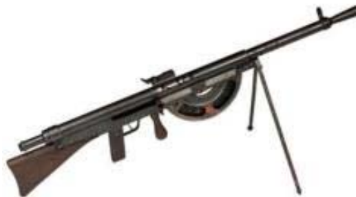
Automatic Rifle Model M1915 (Chauchat) 20 lbs “Marching Fire” concept.
