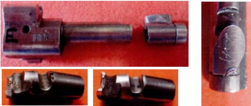
Bolt Assembly replaced at 15K rounds to avoid breaking in front of cam lug.
