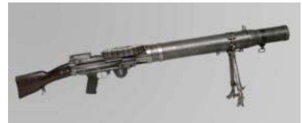
M1914 – Lewis Gun (pan feed) Active Air Cooling @ 28 lbs.
