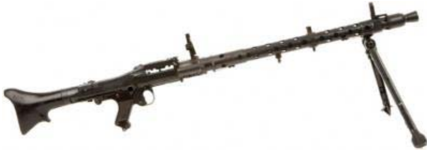
1934 – MG-34 Primary German GPMG entering WW2 and first true GPMG (used in Lafette Mount for Medium MG Role) Select Fire by finger position on trigger @ 26.7 lbs.
