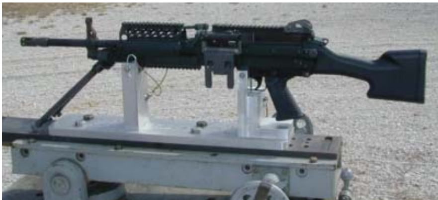
Navy MK48 MOD0 Fixture Mounted Dispersion Test Configuration.
