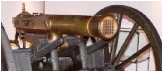
1851 Mitrailleuse -Belgium (service 1866 France)– “Grapeshot Shooter” (multi-bore barrel) 1858 French Rifled field guns not good for Shot.
