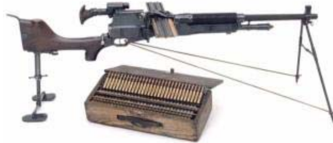
M1909 Benét–Merciè (French Hotchkiss) U.S. LMG entering WW1 @ 30 lbs & 400 rpm cyclic (150 rpm actual) and 6X optic with basic range finding reticle.
