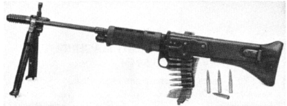
USA T44 - 14 lbs @ 500 rpm – FG-42 Action and MG-42 Belt Feed Evolved into M60 GPMG.
