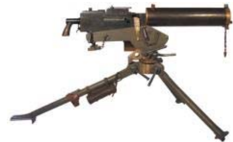
M1917 Browning – Water Cooling provided excellent sustained fire capability -design available from 1910 (considered a Heavy MG at time).
