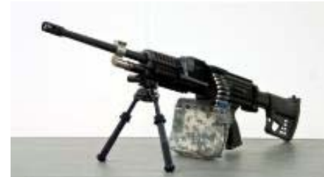
Army LSAT LMG @ 10 lbs w/ Case-Telescoped Ammunition @ 20.4 lbs less than M249 - both with 1,000 rounds.
