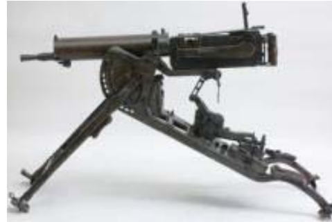
German Maxim MG08 – Cooled with recirculated water.
