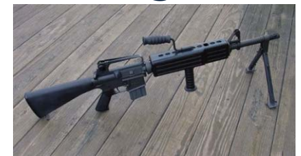
Colt M16 LMG / LSW 5.56X45mm @ 12.7 lbs Open Bolt / Full-Auto only.
