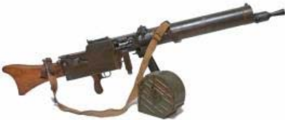
1915 – MG08/15 @ 36-39 lbs (w/ 5 pints water) primary German LMG in WW1 - Adaptation of MG08 Heavy MG – sustained fire capable for up to 6,000 rounds.
