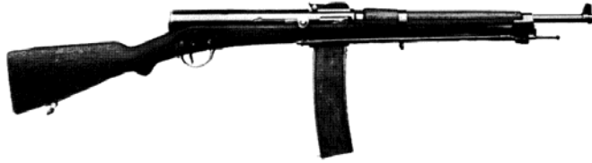
Ribeyrolle AR M1918 - 8X35mm @ 11.2 lbs (blow back 400m range) France - .351 Win. based cartridge.
