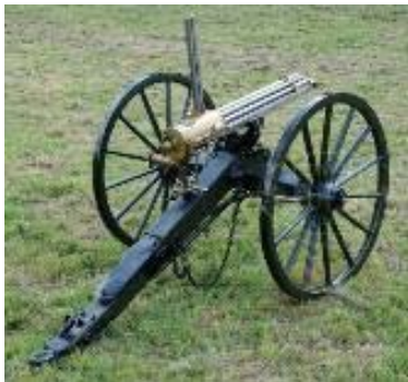
1862 (Pat.) Gatling – Rotary, Single Feed, 1 bolt per barrel.
