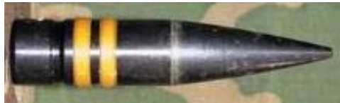
30mm GAU-8 Plastic Driving Bands – should consider for small arms rounds to increase barrel life/ reduce heat & fouling.
