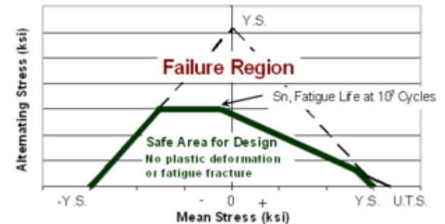
Figure 1. Alternating vs. Mean Stress Diagram Example (Goodman Diagram) for Axial or Bending Loads
