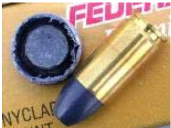
30mm GAU-8 Plastic Driving Bands – should consider for small arms rounds to increase barrel life/ reduce heat & fouling.
