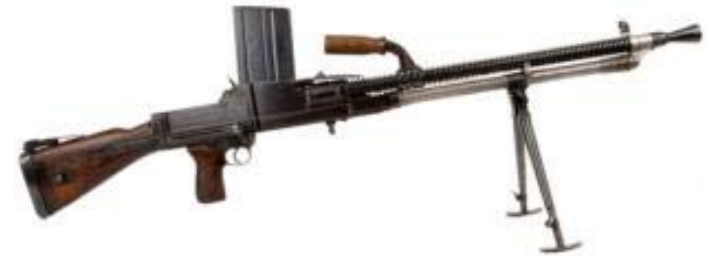
1926 Cz Zb 26 @ 21.3 lbs – Quick Change Barrel.
