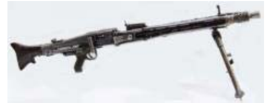
MG-42 7.92X57mm @ 25.5 lbs 1,200-1,500 rpm -Very Suppressive.
