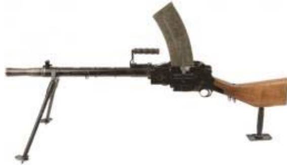
1902/04 Danish Madsen (20 lbs) First true LMG produced in quantity (later model shown).
