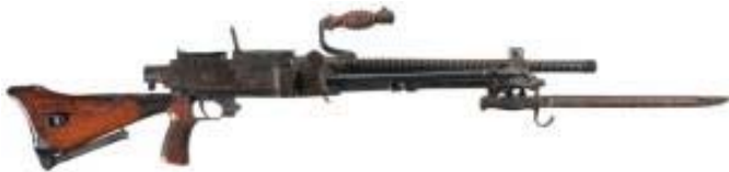
1937 Japanese Type 99 Quick Change Barrel 7.7X58mm Arisaka.
