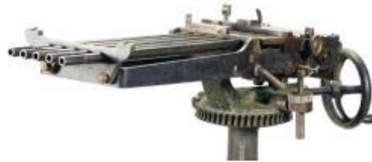
1870's Nordenfelt (Sweden)– linear multi-barrel / toggle feed.
