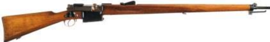
M1894 Mondragon (Mexican/Swiss) – Straight Pull Bolt Action with “Automatic” Mode - fires when bolt is manually cycled without trigger contact.
