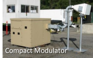
Compact Modulator FY 14 SIZE: 450 ft 3 WEIGHT 4,500 lbs
