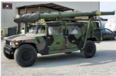
TEAMS Tactical Elevated Antenna Mast System
