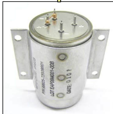
LiSi/FeS 2 Thermal Battery (Device No. G3190B2)
