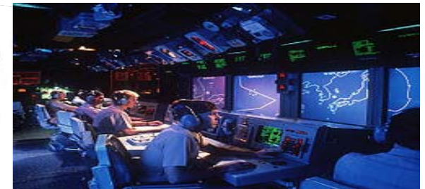
Display system for Aegis-equipped destroyer
