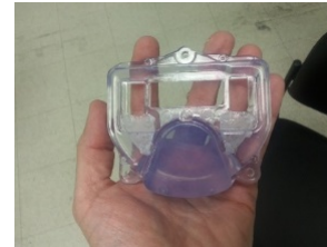
3d printed mockup of next gen vacuum cell for dual atom accelerometer and gyroscope prototype
