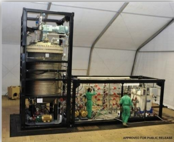
The Field Deployable Hydrolysis System. Developed in only five months, and was deployed on the CAPE RAY and destroyed 600MT of Syrian chemical weapons in 42 days (2014).
