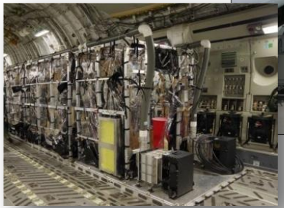
Transport Isolation System, Safely transport Ebola Virus Disease patients, or other highly infectious patients on military cargo aircraft.
