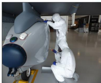
Harvester Particulate Airborne Collection System (PACS). Airborne Debris Collection Following a Nuclear Event
