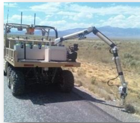
Advanced Ground Sample Collection Platform (AGSCP). Collecting Radioactive Debris Following a Nuclear or Radiological Event
