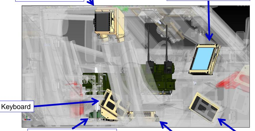
Digital Beachhead Shared Processing Unit (SPU) and Ethernet Switch
