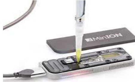
This thumb drive-sized sequencer connects to a laptop, rapidly reads DNA, and identifies genetic material in uncharacterized samples.
