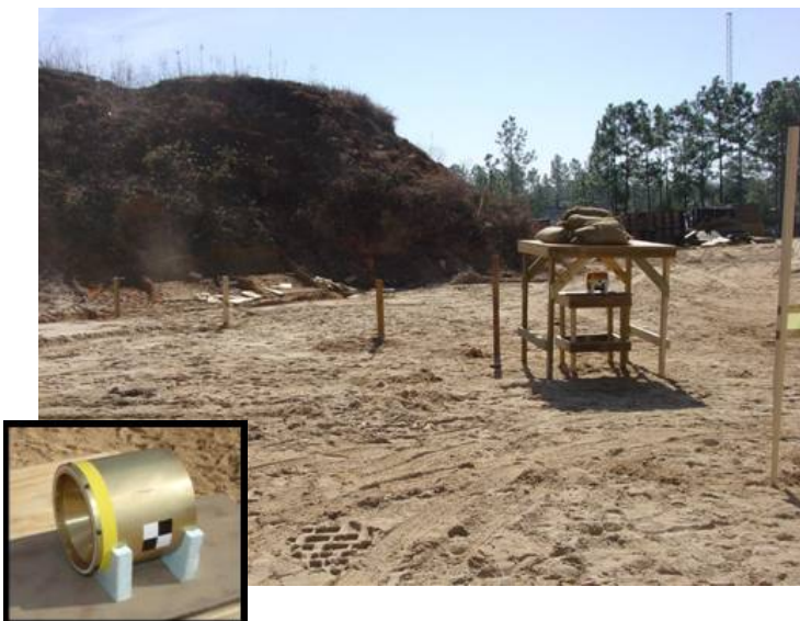
1829 m/s frag impact test setup
