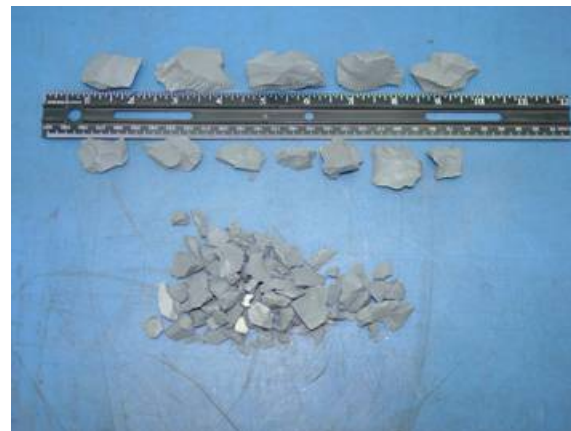
Type 4 test results for PAX-30 showing large case fragments and unreacted explosive
