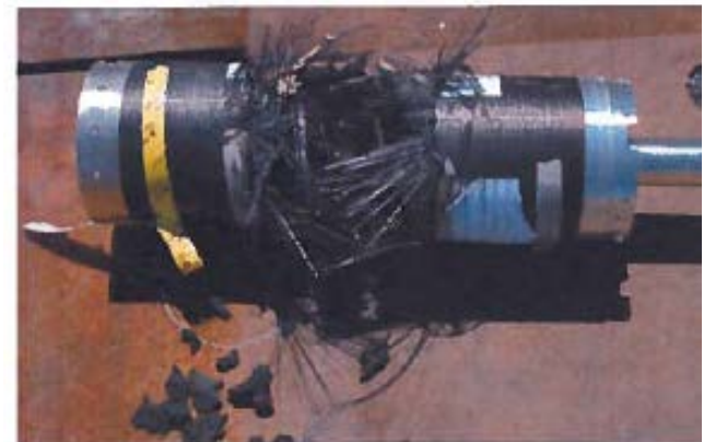
Figure 14 : Fragment impact result with a composite case
