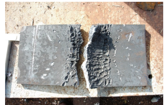
Witness plate after type 1 reaction
