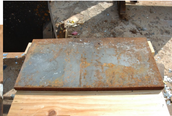
Witness plate after type 4 reaction
