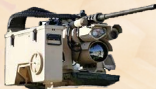
Common Remotely Operated Weapon Station (CROWS)
