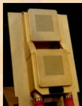
Precision Fire Control Radar (PFCR)
