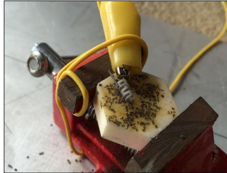
3.2v Rated AlN Heater, 9v DC Transistor Battery, Federal (GD-SMPD) .22LR Rimfire Propellant, Estimated Temperature Rise >300F In Less Than One Second
