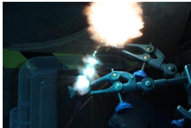
Unlike The Gentle Bursting Of A Light Bulb Or The Puff Of Arcing Wires, AlN Heaters Can Be Made To Instantly And Violently Explode On Overvoltage.
