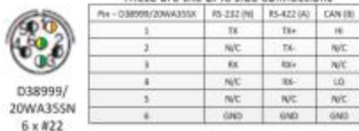
These are the EPIC side connections
