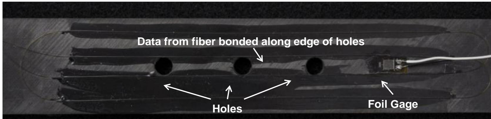
Carbon composite coupon loaded in cantilever beam configuration
