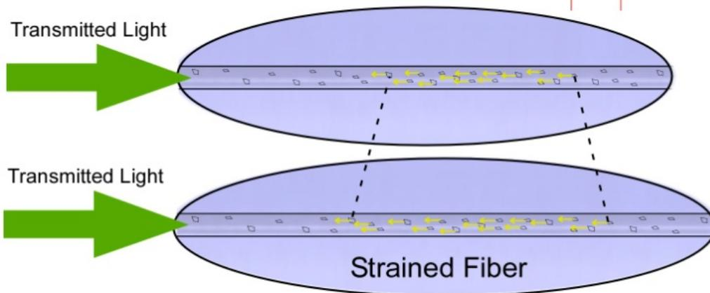
Backscatter Frequency shift correlates to change in applied strain or temperature
