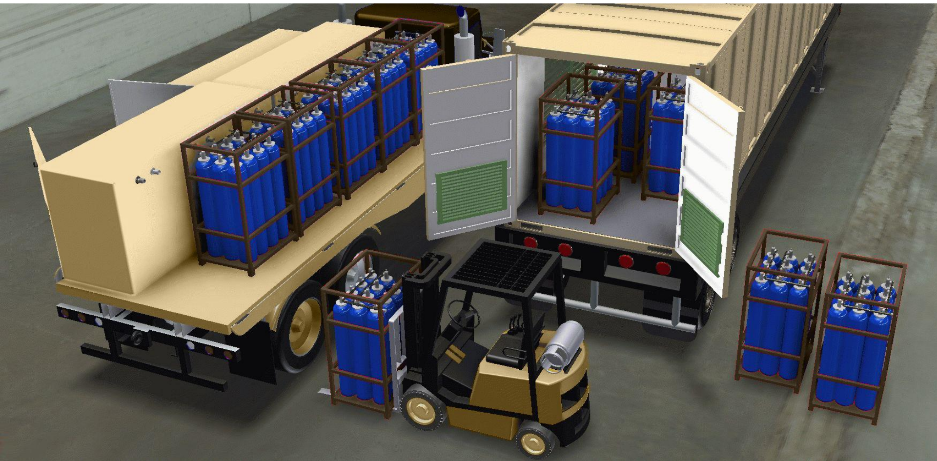
Distribution of H2 Storage Module to Mobile Refueling Vehicle & Permanent Station
