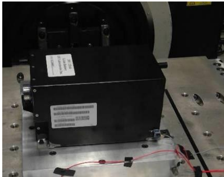
EIC 28V/25Ah battery has passed 1- EMI MIL-STD 461F 2- Aircraft mechanical Shock and Vibration tests 3- Aircraft Electric Power Characteristics MIL-STD 704F
