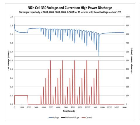
HPPD with variable discharge current pulses and cumulative Ah output at isotherm conditions
