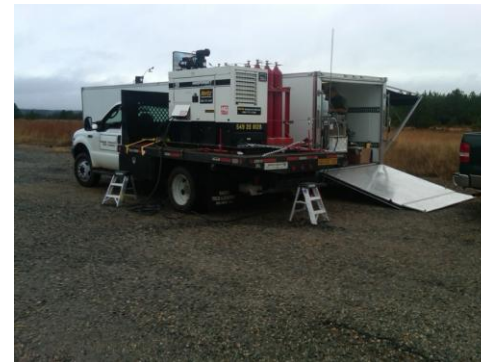
Proton electrolyzer at remote launch site, Fort Benning, GA, December 2012
