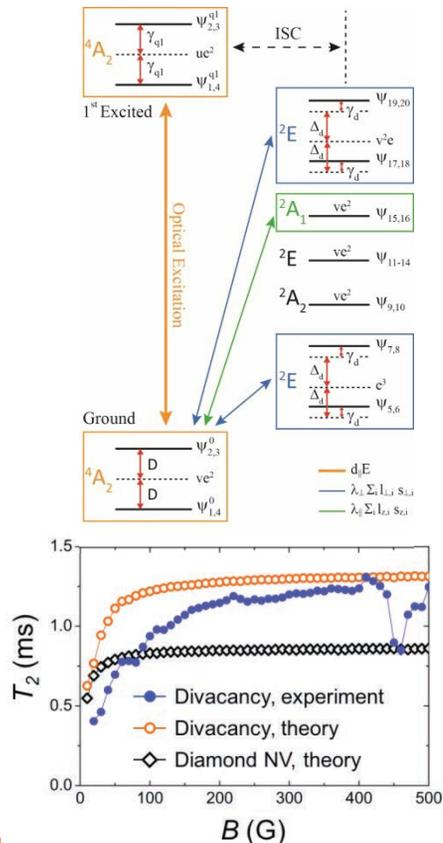
Coherence times of spins are longer in SiC than diamond NV-centers
