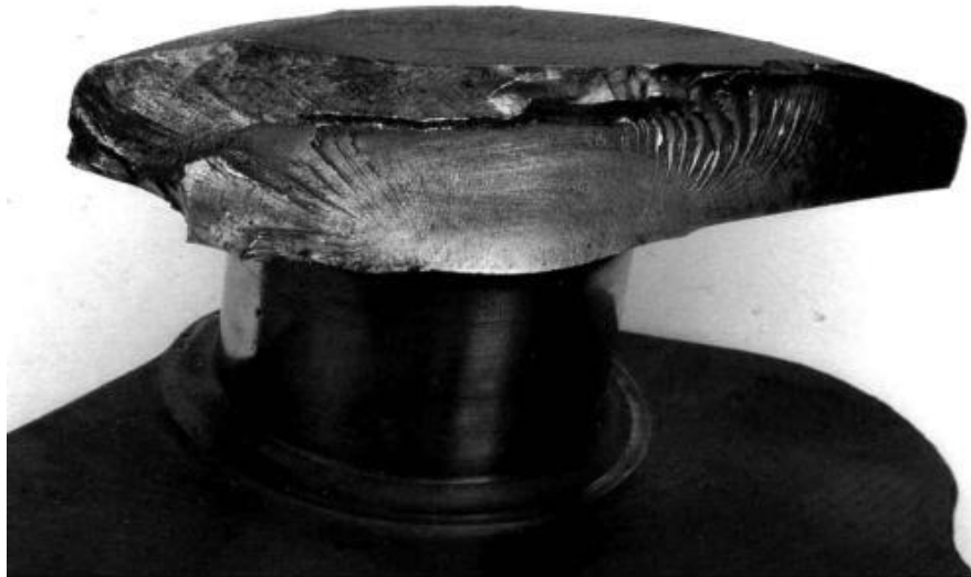
Example of crankshaft fatigue (source: Wikipedia)
