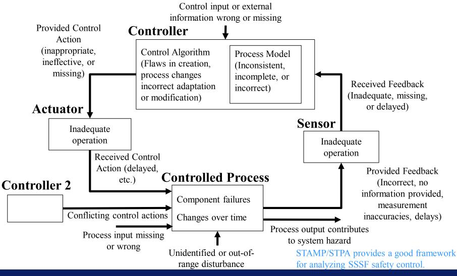
We do not assign a SwCl because in STAMP software can and should be treated in the same way as hardware, i.e., the hazards are identified along with causal scenarios leading to the hazards. Then engineers can eliminate or mitigate those causes according to standard system safety practice and design precedence . . .
