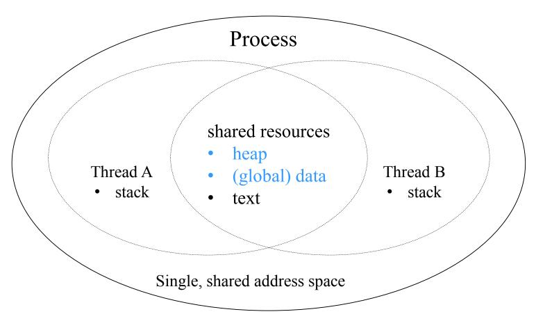
Variables or objects in the *heap* or *data* can be shared by the threads. This can lead to race conditions or thread deadlock. (*Text* can also be shared, but (usually) does not change in
