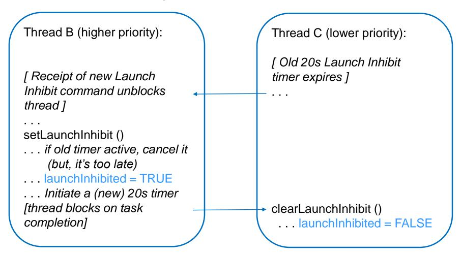
Timer intended to clear OLD Launch Inhibit condition clears NEW one instead!. A data synchronization mechanism should be used to protect the shared data item.
