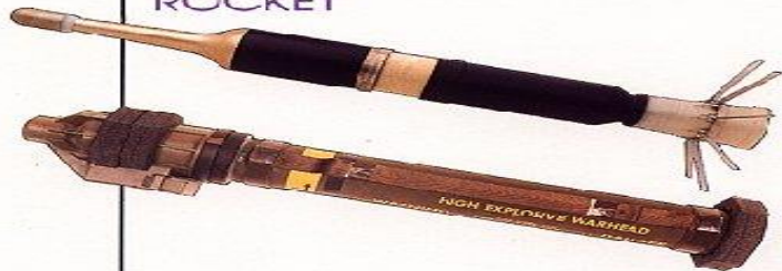
HIGH EXPLOSIVE ANTI-ARMOR (HEAA) ROCKET
