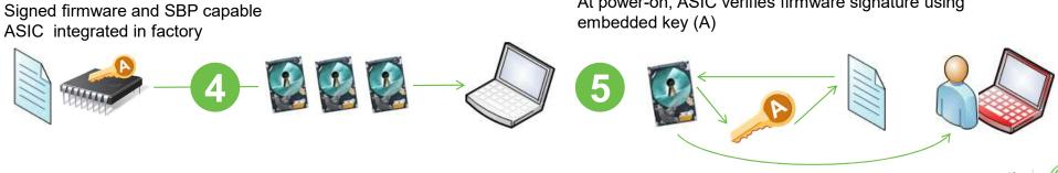
At power-on, ASIC verifies firmware signature using
