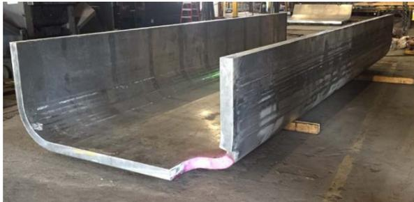
First formed aluminum tracked combat vehicle hull produced
