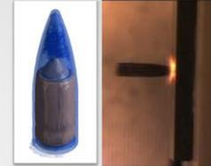
Comprehensive projectile characterization, high-speed video determination of pitch/yaw
