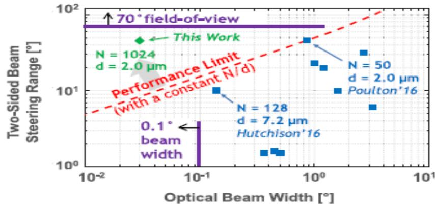
Fig. 2. Design tradeoff between beam-steering range and beamwidth for a constant  $N/d$ , where  $N$  is the number of antennas and  $d$  is the antenna pitch in a uniform optical phased array.
