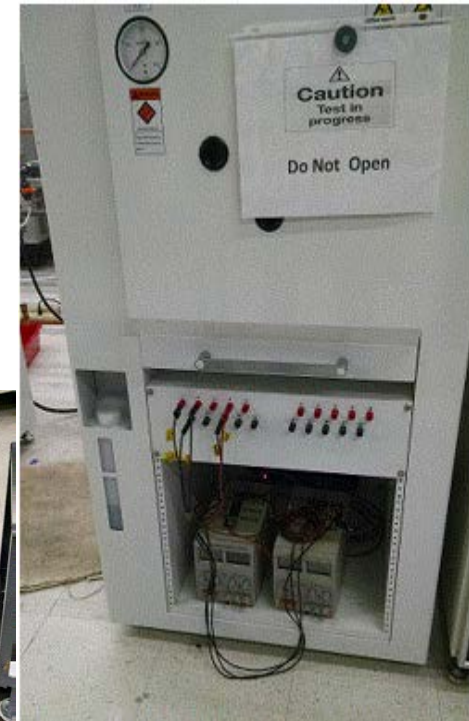
HAST Chamber with humidity control and voltage bias interface. Tested at HASTest Inc.
