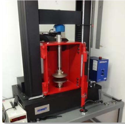
Admet Universal Tester (for compression, confined compression, Brazil tests)
