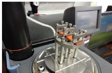
Example DMA Test Configuration
