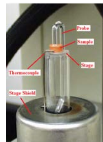
Example TMA Test Configuration
