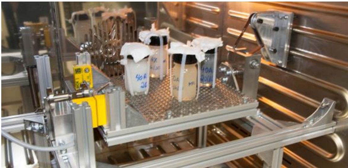
Figure 8: Real photograph of the turning device inside the oven with mounted samples in small glass bottles.
