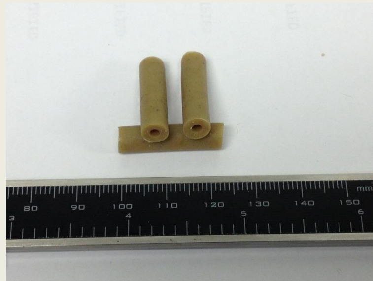
Figure 2: RPD-380 w/BN Single Perf grains used in erosion testing
