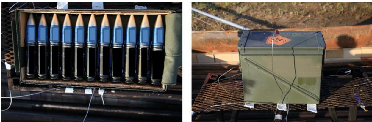
Figure 8. Ammo Can Containing 110 Medium Ammunition Rounds. Shown at Right, Ammo Can on Test Stand Prior to Propane FCO Test in 3.7 m by 3.7 m Burner.
