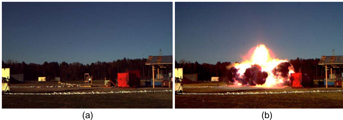
Figure 7 The test article (a) before the e fragment impacted, and (b) the detonative response that followed after impact.
