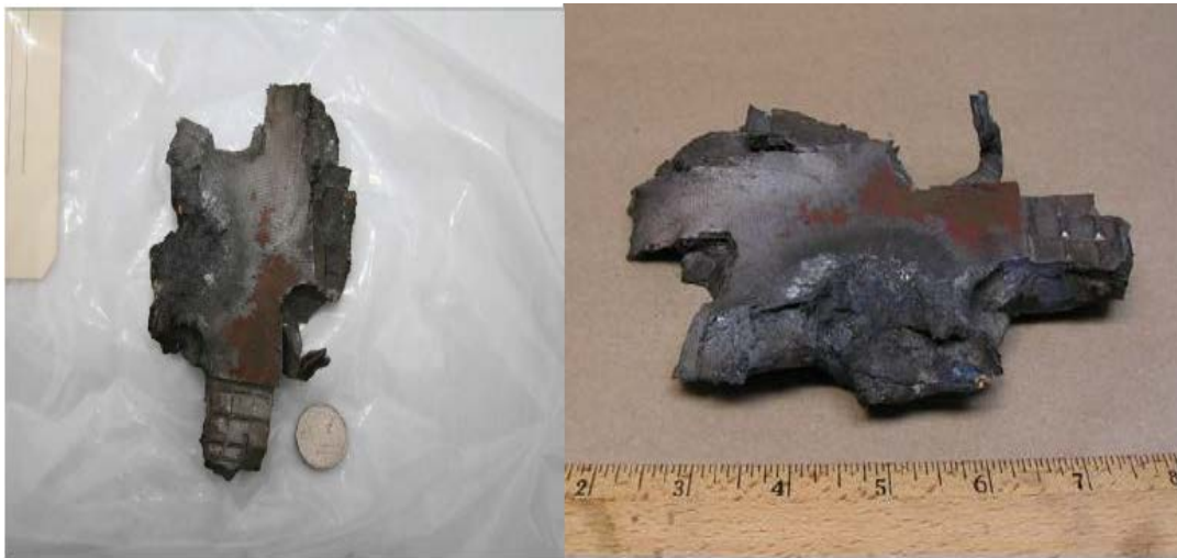
840 g steel fragment from a M107 155 mm artillery shell that reached 1824 m after a sub-detonative response.
