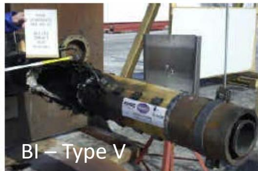
IM Tests on the ESSM Motor featuring a carbon fiber reinforced composite material\*
